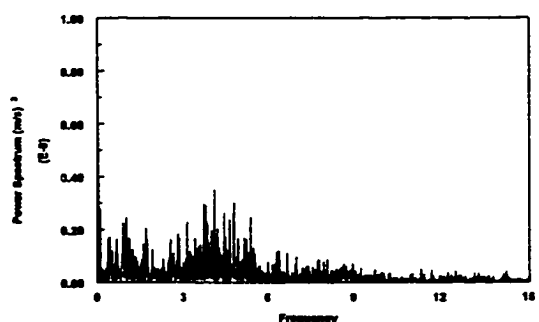
Figure 4.3.15-g Power spectrum of the instantaneous mass transfer coefficient at V_{sl}=1.2 m/s and V_{sg}=2.4 m/s in water/gas flow
